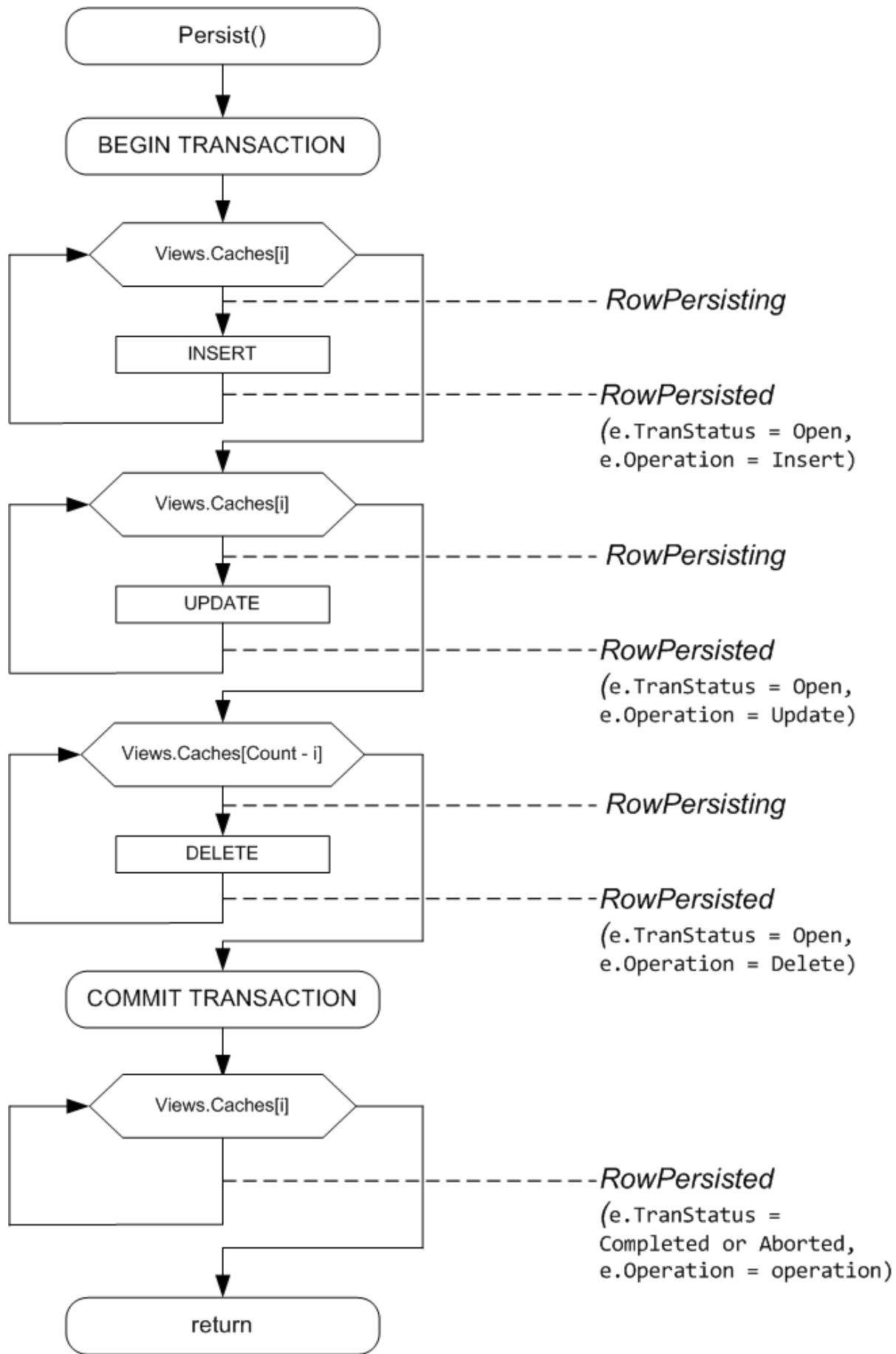
Figure: The process of saving changes from cache objects to the database
